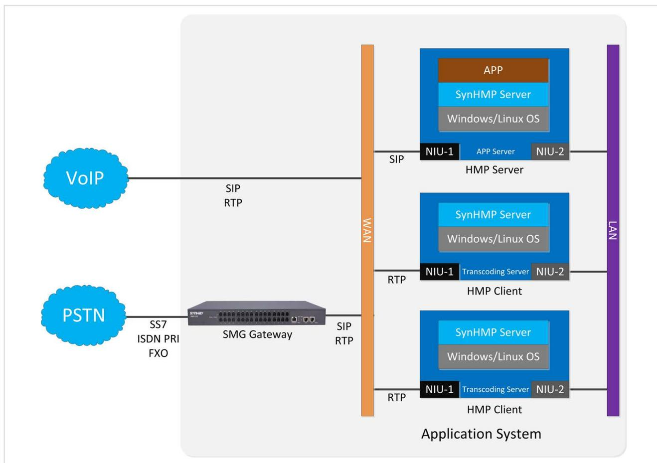
SynHMP consists of two parts: HMP Server and HMP Client. HMP Client receives and transmits the RTP data from/to HMP Server and the remote point, besides performing data encoding and decoding. HMP Server is to record the received RTP packets and write them to the hard disk, read the voice data from the memory or the hard disk, package them into RTP and transmit it to HMP Client. At the end, HMP client sends the RTP to remote point.
